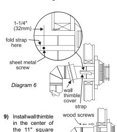
and attach with wood screws (Diagram 7).
